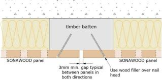
Face fix with countersunk screws to Rondo KEY-LOCK  $^{\footnotesize\text{\tiny{\$}}}$  furring channel/batten
